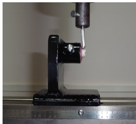
Figure 2: Shear load testing carried out in INSTRON 3366 with the specimen attached to the fixture
