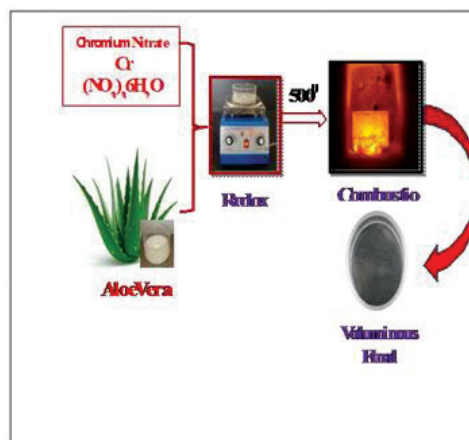
Fig. 1: Flow Chart for Preparation of \text{Cr}_2\text{O}_3 NPs
