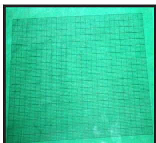
Fig- 1 Transparent flexible grid with smallest square measuring 1 mm 2 .
